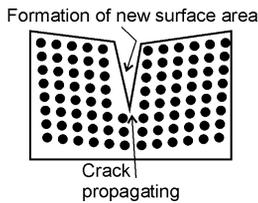
**Fig. 11.4** Crack propagation in brittle fracture
