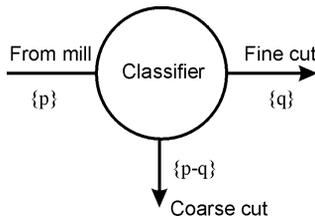
**Fig. 11.8** Schematic representation of a classifier
