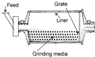
**Fig. 11.11** Illustration of a ball mill with an attached grate discharge to retain balls and oversize material
