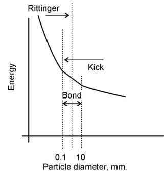
Fig. 11.5 Crushing laws
