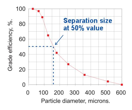
Plotting mid-points against grade efficiency for each grade gives a separation size of 160 microns.
