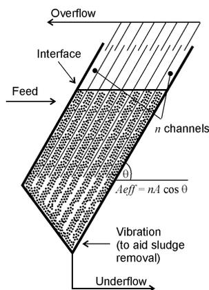
Fig. 6.17 Lamella separator or thickener - has lots of sedimentation channels in parallel
