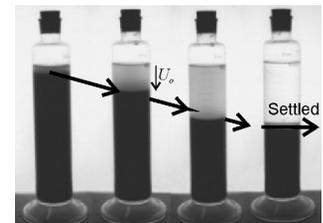
Fig. 6.2 Hindered settling in cylinders - interface fall with time
