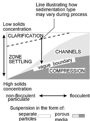
**Fig. 6.14** Diagram showing types of sedimentation
