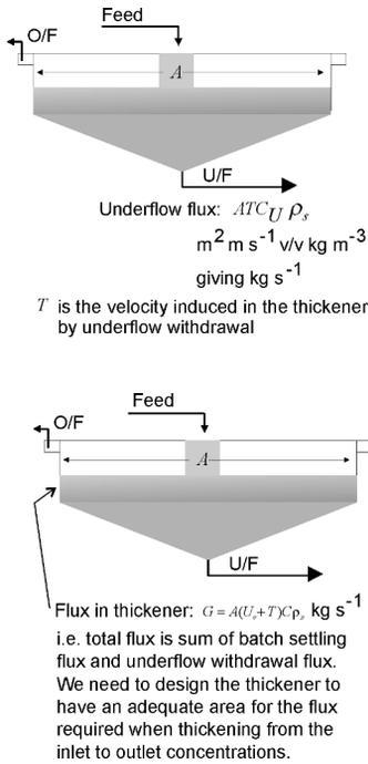
Fig. 6.8 Fluxes in a thickener
