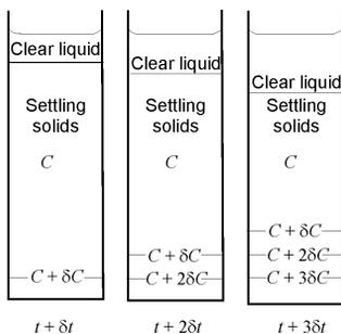
**Fig. 6.4** Solid concentration increases starting at the base and apparently rising upwards in the vessel
