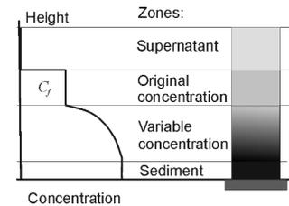
Fig. 6.5 Zones within a settling suspension at a selected time  $t$
