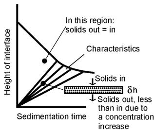
**Fig. 6.13** A lamina layer within a settling suspension and the batch settling curve
