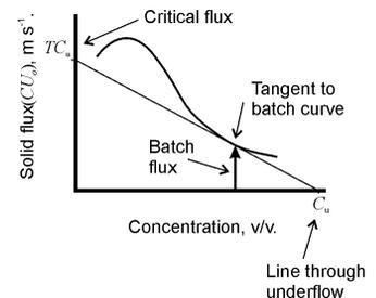
Fig. 6.12 Construction to determine the critical flux - equation (6.8)
