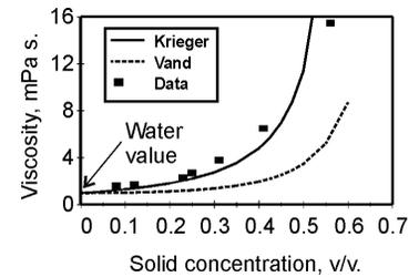
Fig. 6.15 Comparison of Newtonian viscosity equations correcting for solids presence and experimental data
