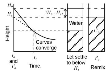
Fig. 6.7 Construction to transform a settling curve
