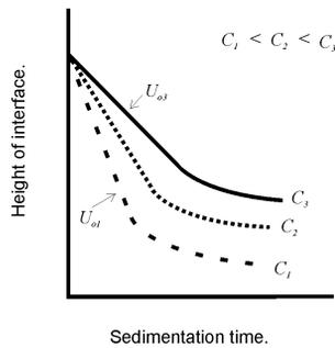
**Fig. 6.3** Variation of settling velocity with starting concentration
