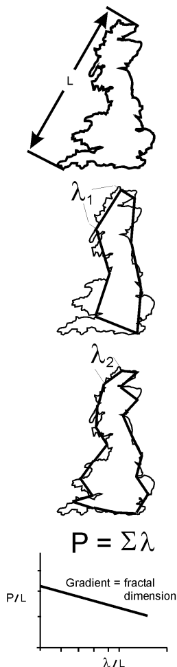
Fig. 2.12 Fractal analysis of a particle: perimeter increases with smaller step sizes ( \lambda ) –rate of increase in perimeter against decreasing step size gives the fractal dimension. Maximum particle dimension normalises step size and perimeter.
